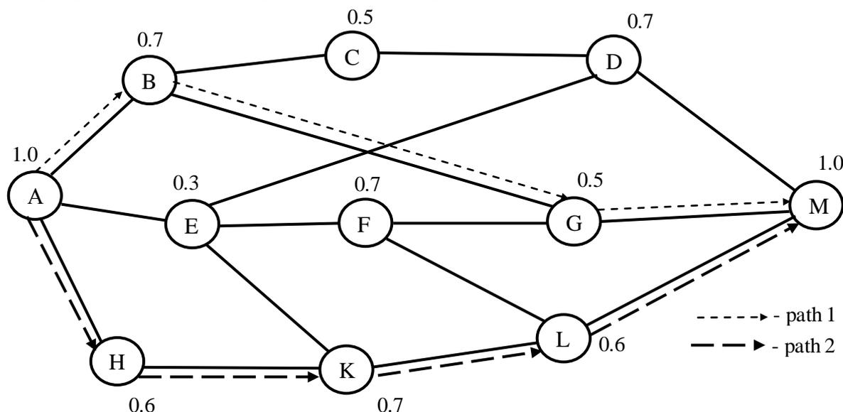
**Fig. 1.** The topology of the DCS with the predefined trust levels for nodes actions
