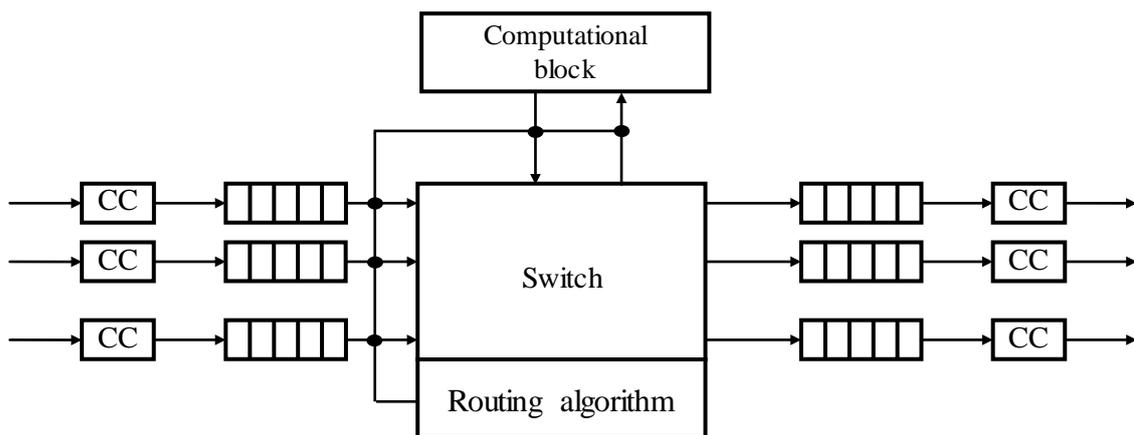
**Fig. 3.** The generalized structure of a router for the distributed computer systems and switched networks This router performs the data processing and transmitting in 4 phases [3,4]:
