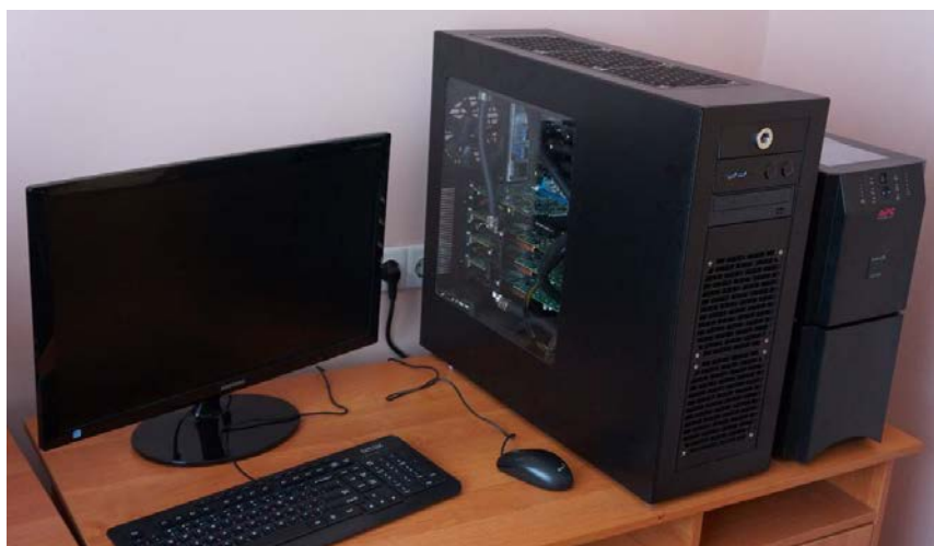
Fig. 1. Personal hybrid computing system based on graphics processors
