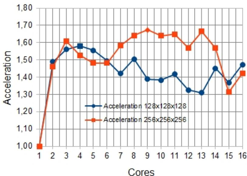
**Fig.3** Acceleration dependences from number of CPU cores (HPCG cluster, Linux)
