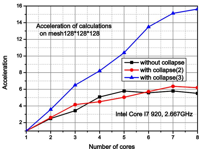
Fig.1 Intel Core I7 920, acceleration for computational grid 128x128x128
