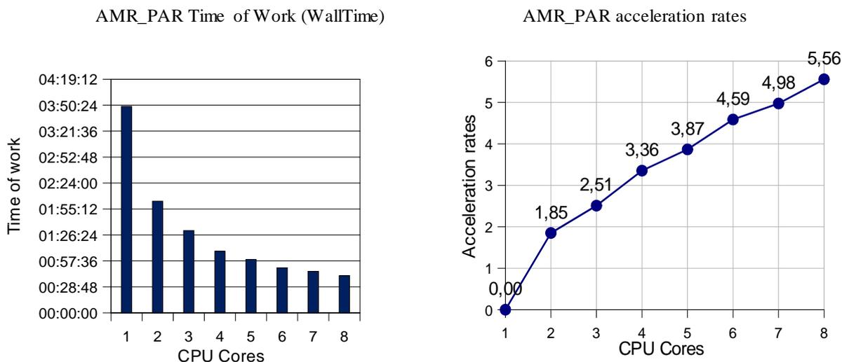
**Fig.2** Intel Xeon E5310, acceleration for computational grid 128x128x128, MS Windows
