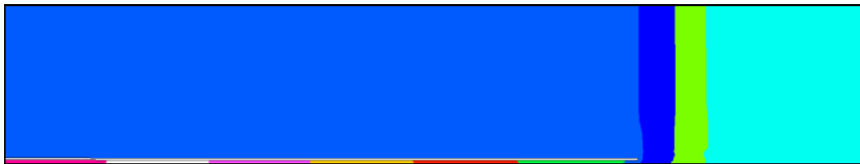
Fig. 2. Example of METIS decomposition into 10 parts of the typical computational domain for 2D axisymmetrical internal and intermediate ballistics calculation
